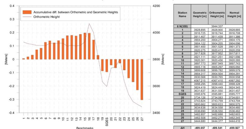
The following charts and tables show the differences between Orthometric and Ellipsoidal Heights and the difference between IGN N and EGM08 N:
